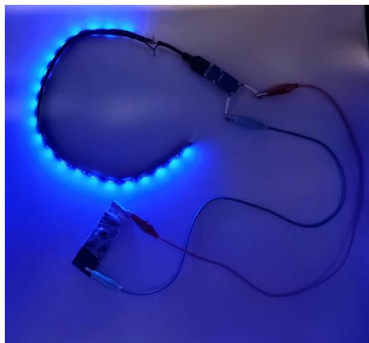
Supplementary Fig. 40. Photograph of a wristband with LED lights powered by the flexible solid-state ZAB with Fe,W-N-C catalyst as the air cathode.
